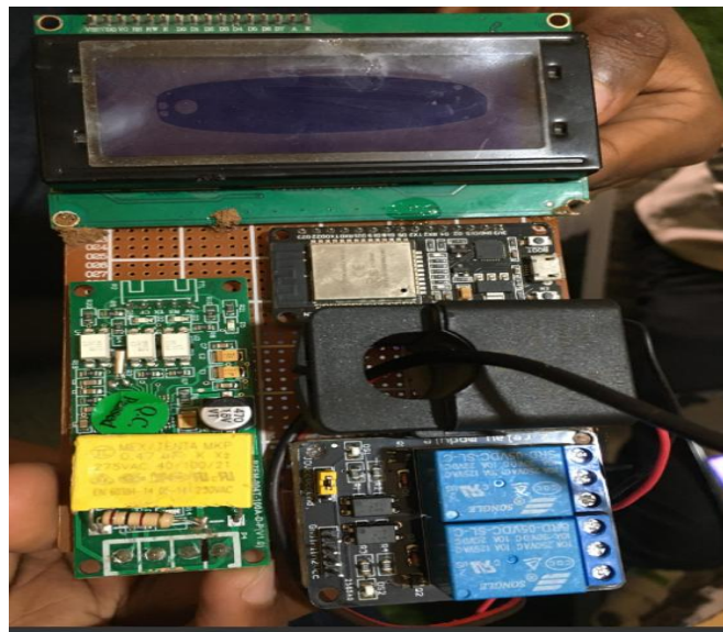
Figure 13. Final assembled smart energy meter circuit on Vero stripboard
