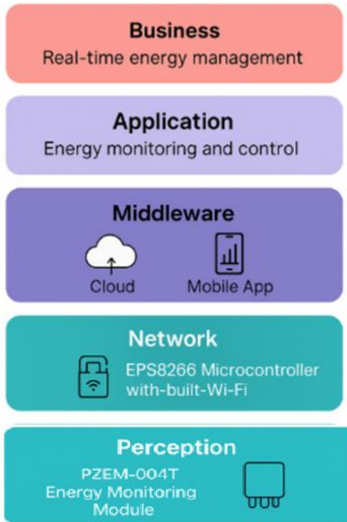
Figure 9. Layered IoT Architecture for Smart Energy Monitoring System [64]
