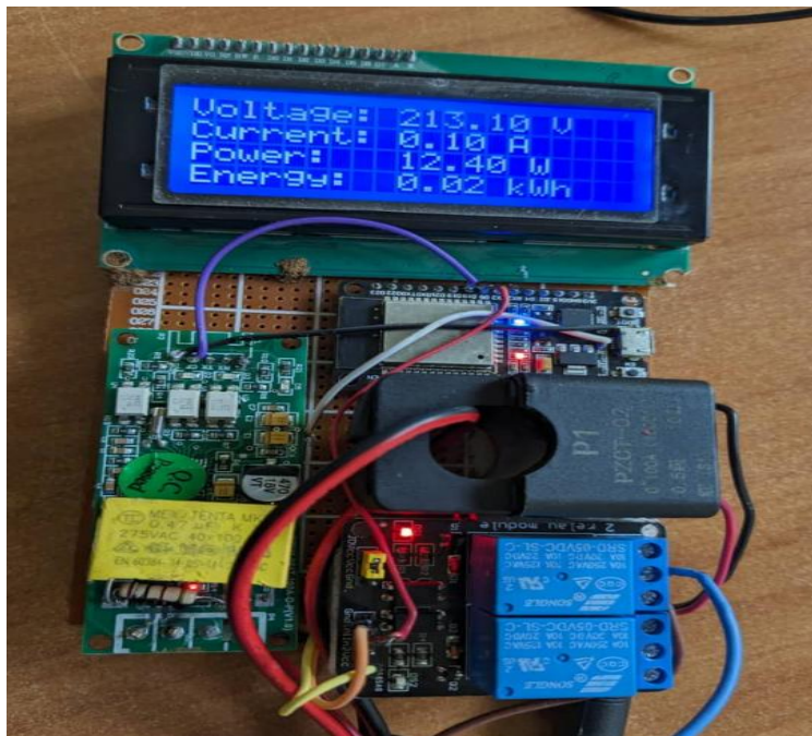
Figure 18. Smart meter displaying 0.02 kWh after extended runtime
