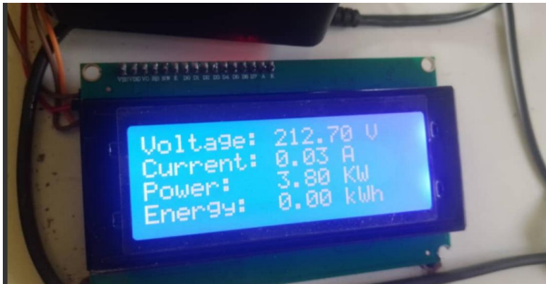
Figure 19. LCD display photo during live readings (to show onsite real-time monitoring)
